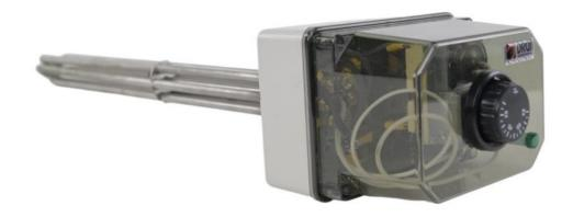
The heating unit is made of stainless-steel alloy AISI 316L (EN 1.4404) and is embedded on a mounted brass cap G  $1\frac{1}{2}$ ". Features a 3-phase thermostat which is externally regulated, a 3-phase safety cut-out with *fail-safe* technology, an indicative bulb, and a safety cover box. It is suitable for enameled and stainless-steel boilers, but not copper or copper-lined tanks.
