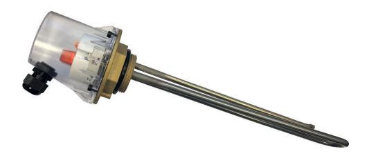
Single phase immersion heater for floor standing boilers on a G 1½" or G 1 ¼" brass flange. A robust and waterproof construction, composed of high-grade stainless steel. The heating unit features a bi-polar thermostat with safety cut-out, a protective transparent polyamide cover, an indicative bulb, and a cable gland. It is suitable for outdoor use (IP67) and is resistant to rain and UV radiation.
